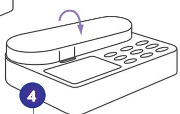
**4** Close the pump door - you should hear a small click when it is closed properly. The pump is now ready to be switched on.
