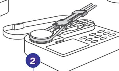
**2** Position the looped section of the silicone tubing around the rotor.
