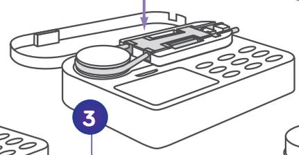
**3** Stretch slightly to seat the cassette into the pump.
