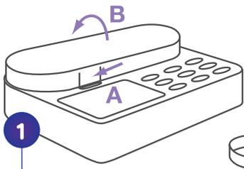
**1** Open the pump door by pressing gently up on the lower wall (A) and rotating the door upwards (B) at the same time.
